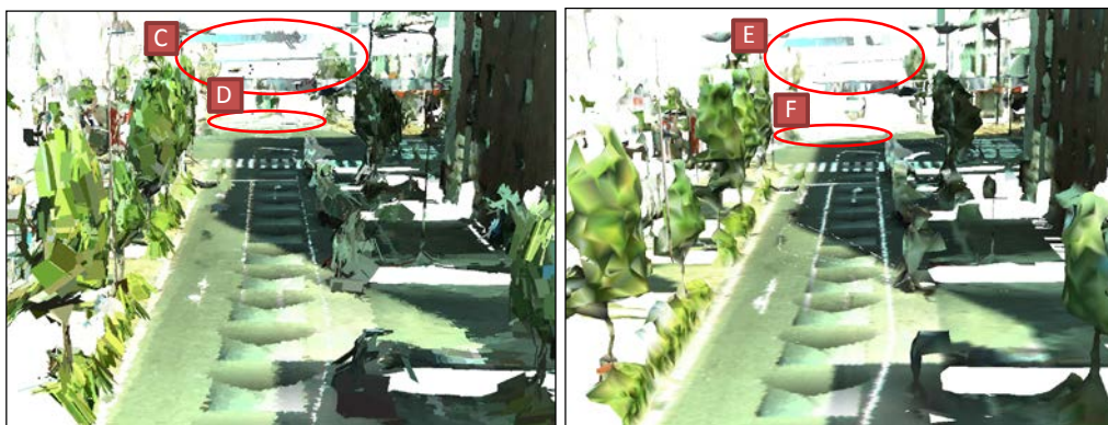
(e) Rendering by splats without point classification (f) Rendering by mesh without point classification (Ball Pivoting [2])
