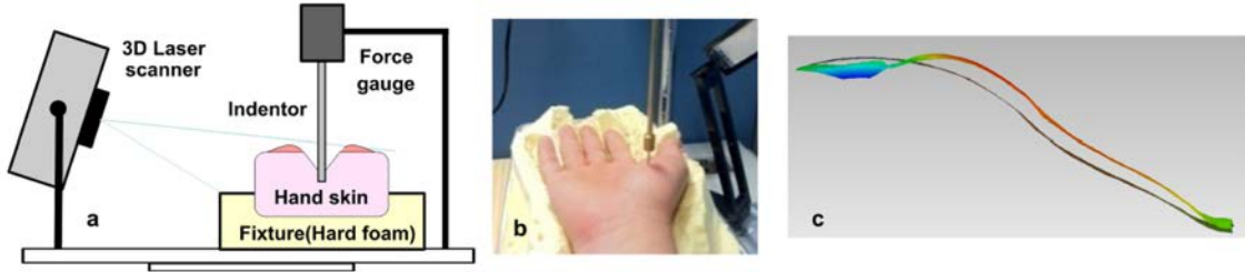
Fig. 6. Indentation test: (a) experimental setting, (b) real scene, and (c) a cross section of 3D deformation map (Geomagic).
