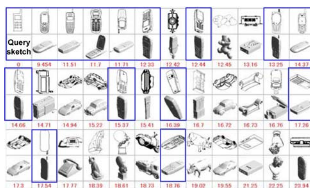
Fig. 17 A result of retrieval for Fig. 13b using GFD and rearrangement using LBP
