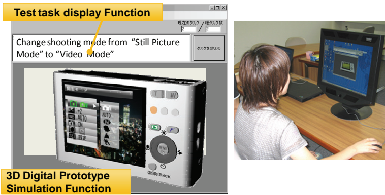
Figure 7. 3D digital prototype simulation function and test task display function.
