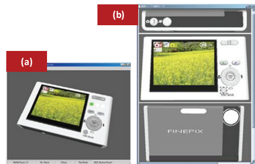
Figure 12. 3D digital prototype (a) and 2D UI software prototype (b).
